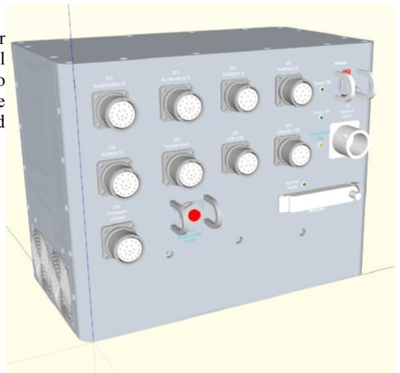
Illustration 1: Proposed preliminary design of Payload Data Router
